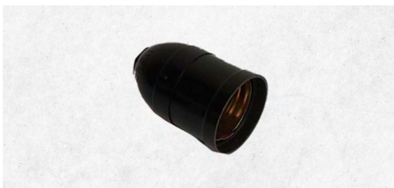
Socket E27 c/roscapara niple de 1/8" NPT 6A-250V bakelita
